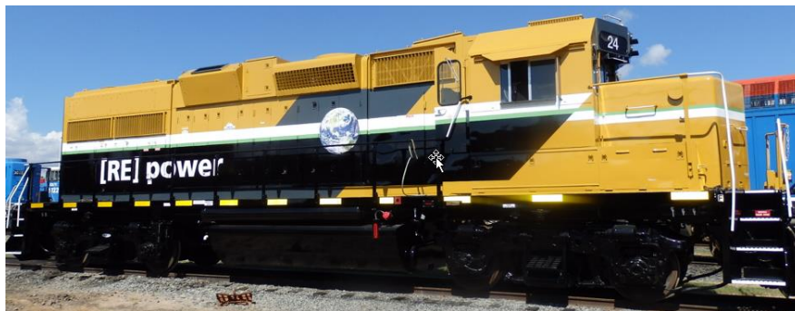
Remanufacture Switch Locomotive EMD24 to Tier 4
